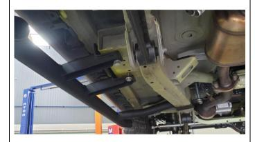
5. Install fasteners into rear mount by hand as shown
