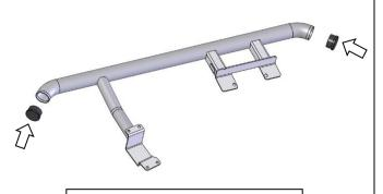
Install Rubber Plugs into both ends of the Rock Sliders as shown.
