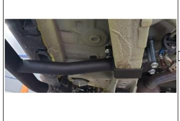
4. With the aid of somebody holding the rock slider in place or the use of axle stands, install fasteners into the front mount by hand as shown
