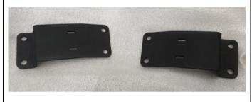
Identify 3752394 L&R. These will need to be positioned on top of chassis prior to fitting Rock Sliders
