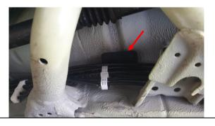
3. Slide brackets between chassis and floor of vehicle in the positions shown. Note the RHS bracket hangs over the brake lines (on RHD vehicles)
