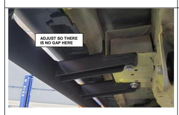
6. Tighten all bolts to specified torque. When tightening the rear mount, ensure that the vertical face is hard against the chassis as shown.
